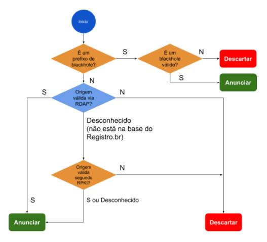
The diagram below outlines how the filters will be implemented in the LONG term.
